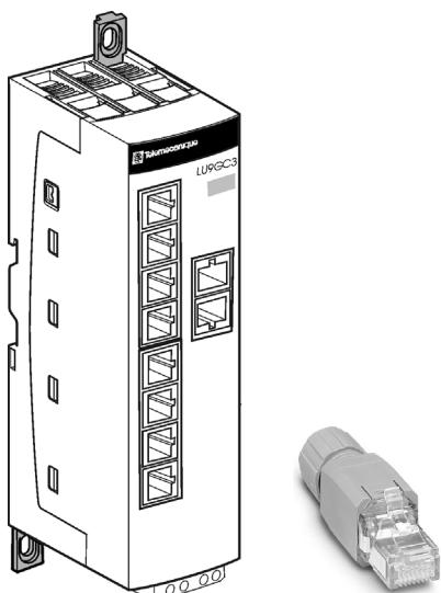
When no Modbus T-adapter is used, please ensure that only the three pins 4, 5 and 8 at the RJ45 connector of the bus connection are connected. Using the PHOENIX CONTACT VARIOSUB RJ45 QUICKON connector is a simple and capable solution to establish a connection between the bus subscriber and the Modbus splitter.
