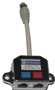
The Modbus T-adapter provides two RJ45 sockets for further bus wiring. On both sockets, which are connected in parallel, only pins 4, 5 and 8 are connected so that also pre-assembled cables (1:1 connection) can be used.
