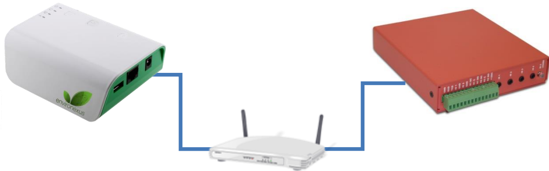
Figure 1 - Connecting Environexus Bridge and Push PC4 to a router
