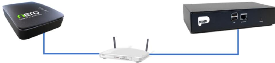
Figure 1 - Connecting Nero Bridge and Push PC4 to a router
