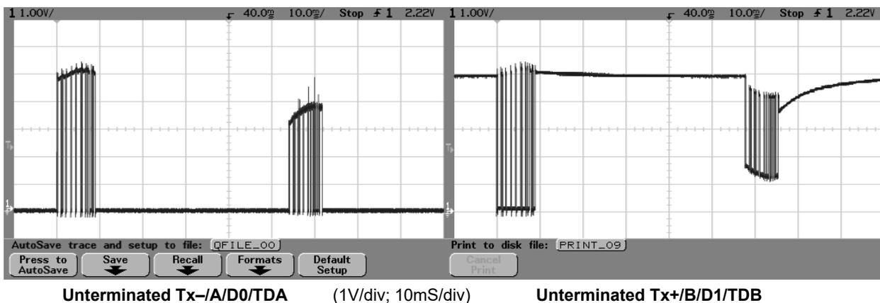
These scope shots were taken with a B&B Model 485BAT3 converter, port powered, connected as described, to an AP9635/41/43/44. Comment: One can see that the B&B converter is using 5V logic (signal swing peak is  $+5V$ ) and the AP9635/41/43/44 uses 3.3V logic.
