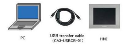
(1) Connect your PC and the GP unit of SP5000 series with a USB transfer cable. If the driver of the cable has not been installed on you PC, a dialog box will appear.
