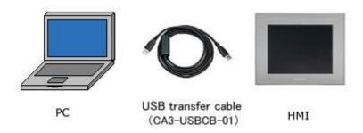
(1) Connect your PC and GP3000 Series with a USB transfer cable. If the driver of the cable has not been installed on your PC yet, a dialog box will appear. Please follow the instructions.
