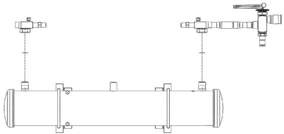
2) Mount the rear support leg to the tank using the 3/8" bolt and hardware provided.
