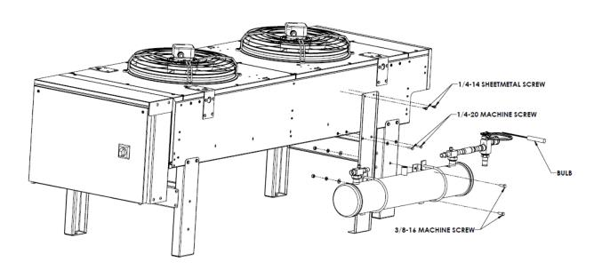
3b) For 800mm units, mark and drill 3/16" pilot holes for the two sheet metal screws. Do not drill more than 3/8" into the units casing. Further drilling may damage the coil. Secure the freestanding leg using the provided sheet metal screws.
