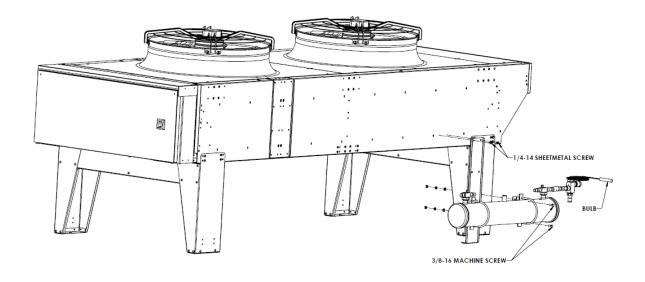
4) Insure that the receiver tank has been installed level position. Failure to do so will cause the system to malfunction.
