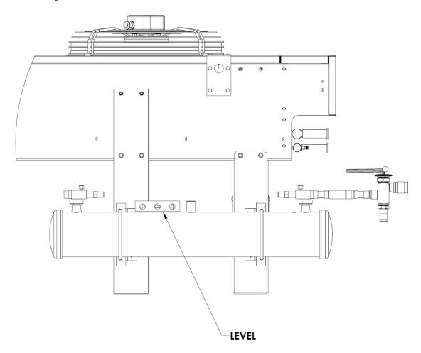
5) Strap the bulb located on the LAC valve to the outlet header of the condenser using the provided strap.
