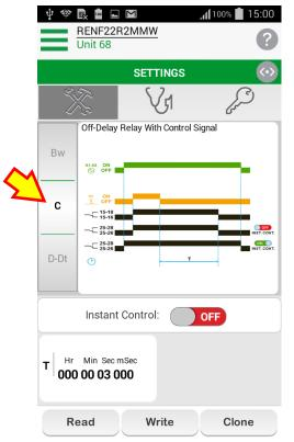
Step 2.1 Function selection Select the Function C. Off-delay relay with control signal
