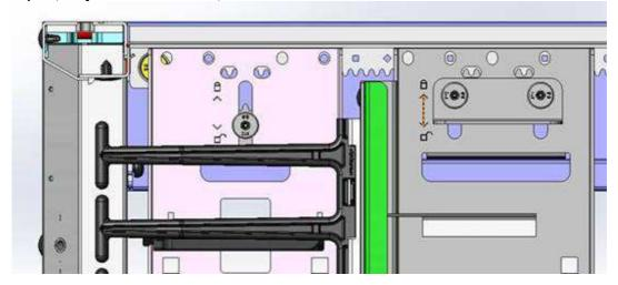
Top-Down View of Cable Fingers with One Accessory Mounting Rail Installed, and AR7540 (1st orientation)
