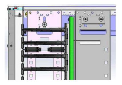
Inside View of Cable Fingers with One Accessory Mounting Rail Installed, and AR7540 (2<sup>nd</sup> orientation)
