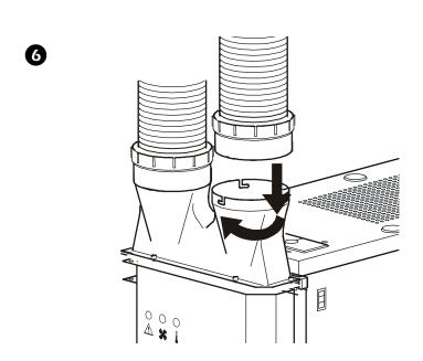
Duct Kit for the Rack Air Removal Unit
