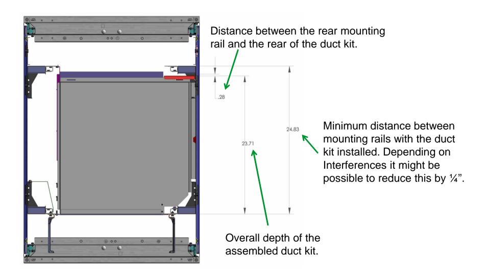
Note: the duct kit needs to be mounted below the chamfered flange on the mounting rail. This will help minimize the overall distance between the front and rear mounting rails.
