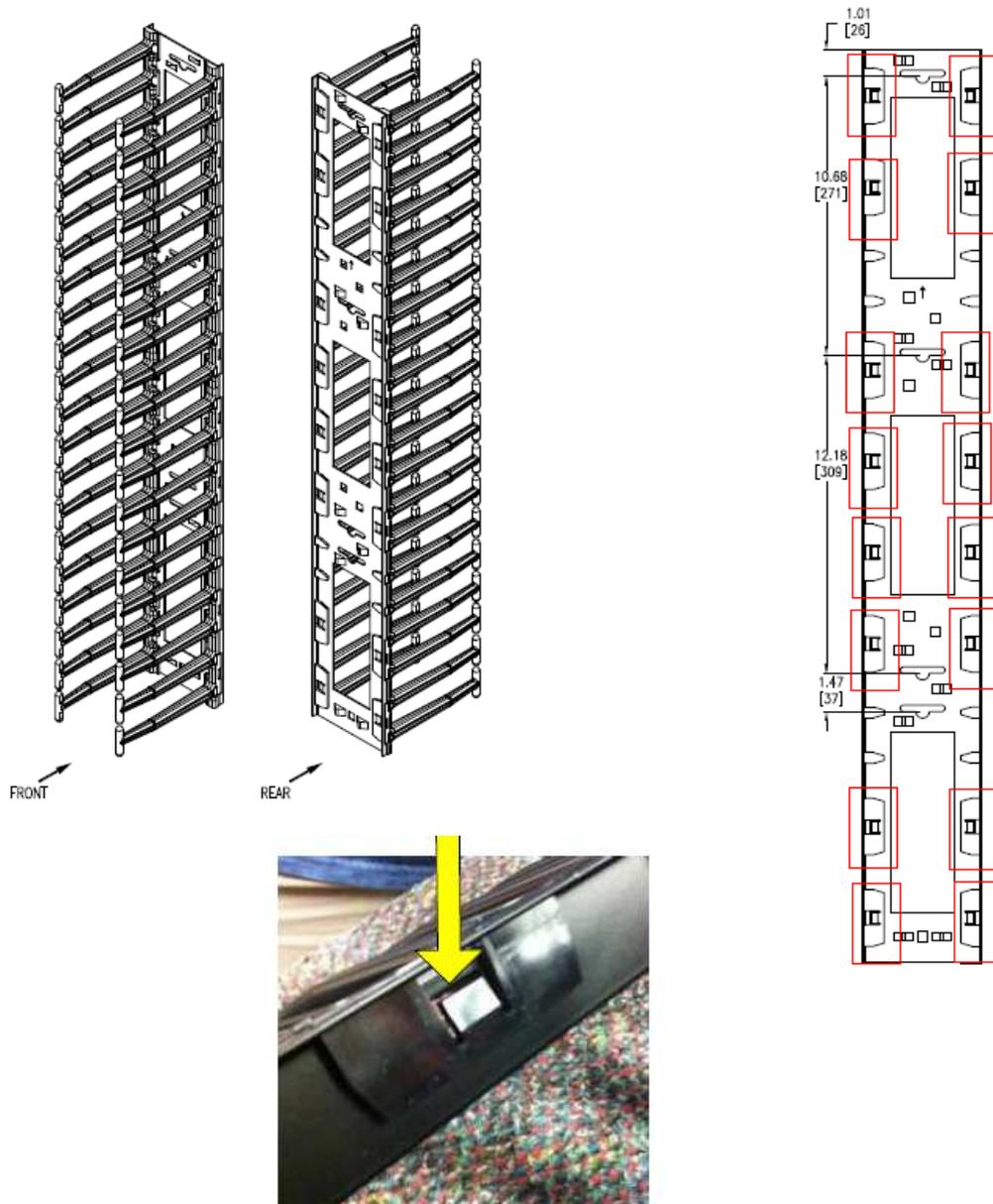
2. Gather the (8) 10U sections of cable guides from AR7721 and reinstall them on the (2) backplates of the AR7580As.
