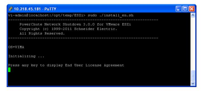
The command used is sudo ./install\_en.sh Further information on the installation PCNS can be found in Kbase articles FA159780 Install PowerChute Network Shutdown 3.0.1 on ESXi 5.0 with vMA 5.0 FA159765 Installation of PowerChute Network Shutdown version 3.0 on VMware ESXi - vMA 4.0, 4.1
