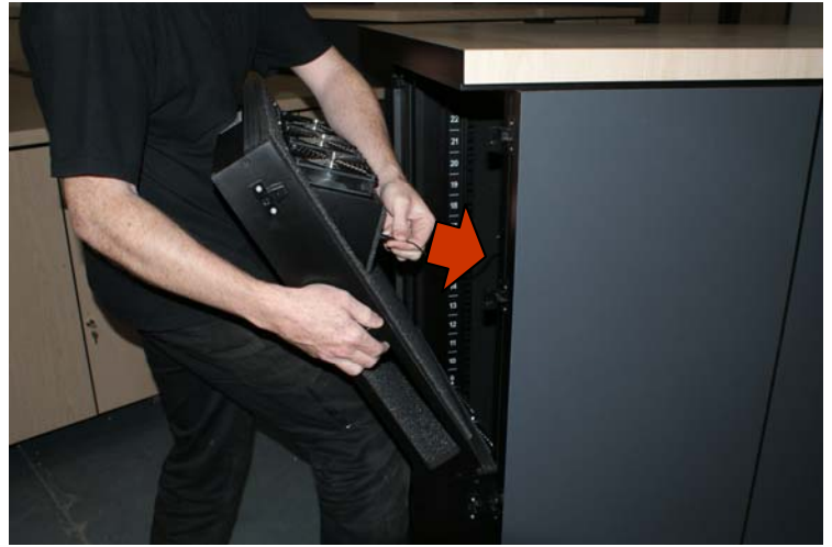
2. Disconnect the DC power jack and remove the FanModule completely.
