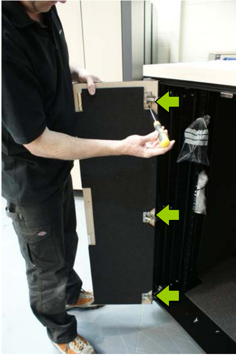
1. Remove the two screws holding each hinge to the door, starting at the bottom and working upward
