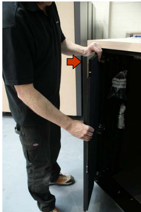
5. Align the hinge-holes on the new door to the hinges and push these together, starting at the top.
