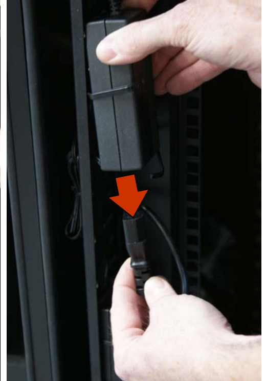
3. Disconnect the PSU
