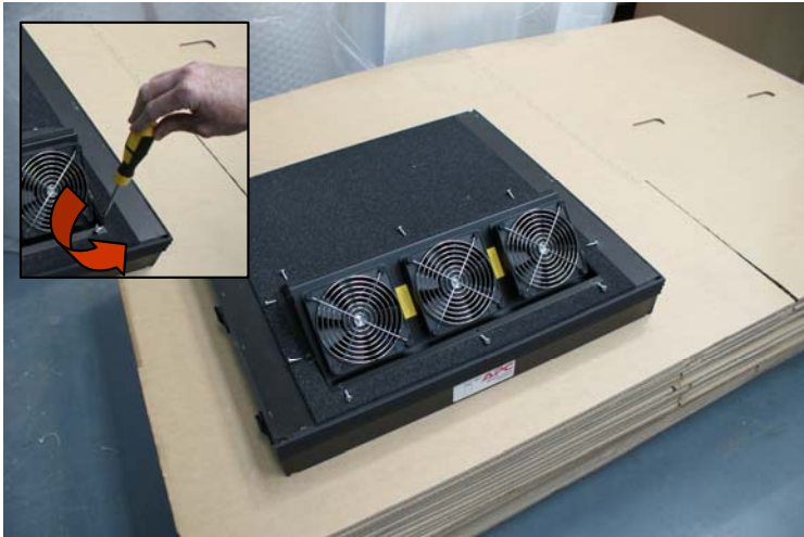
3. Undo the screws holding the FanTray in place.
