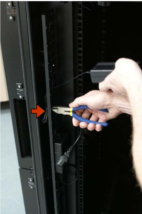
4. Snip the cable-tie holding the jack cable.
