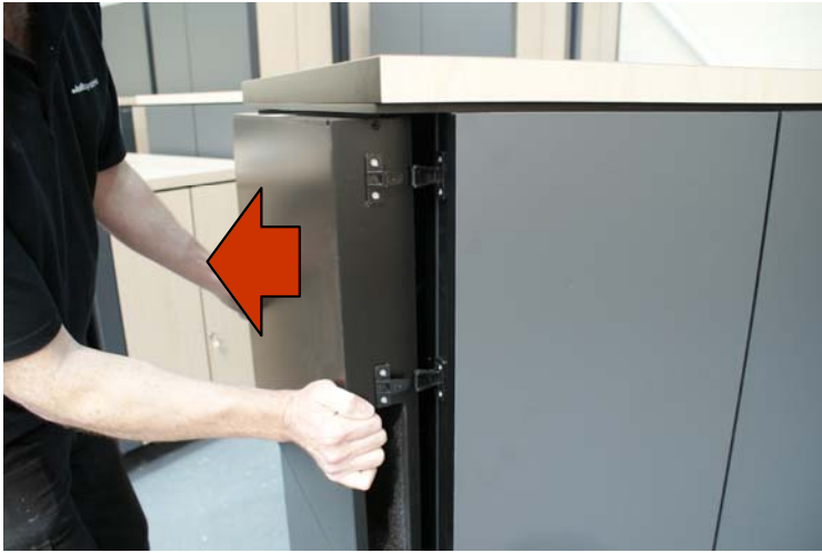
1. Pull the FanModule directly off the rear of the cabinet carefully.
