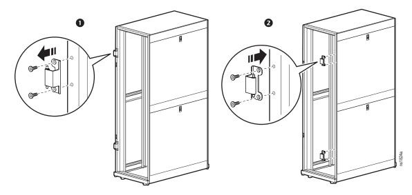
4. Remove and reinstall the hinges in the door frame.
