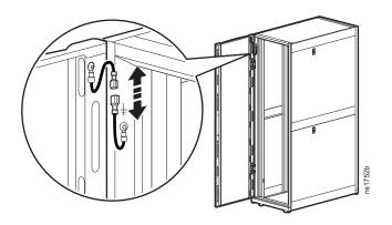
3. Remove and reinstall the hinges on the enclosure frame.
