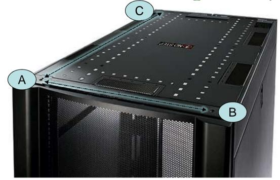
A to B, 600 mm wide cabinet = 487.16 mm center to center A to B, 750 mm wide cabinet = 637.16 mm center to center A to C, 1070 mm deep cabinet = 946.0 mm center to center A to C, 1200 mm deep cabinet = 1076.8 mm center to center
