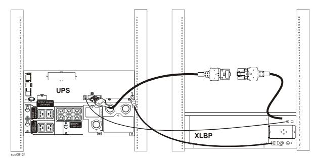
One UPS and one external battery pack and external battery pack extension cable connection. See "Connections" on page 2 to secure the five meter extension cable connector to UPS/XLBP and secure the ground cable connections. Connect the communication cable.
