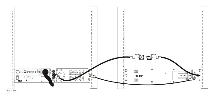
One UPS and one external battery pack and external battery pack battery/communications extension cable connection. See "Connections" on page 2 to secure the five meter battery/communications extension cable connector to UPS/XLBP and secure the ground cable connections.
