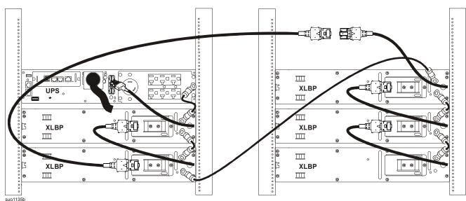
One UPS and five external battery packs and external battery pack battery/communications extension cable connection. See "Connections" on page 2 to secure the five meter battery/communications extension cable connector to UPS/XLBP and secure the ground cable connections.
