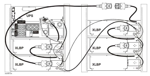
One UPS and five external battery packs and external battery pack extension cable connection. See "Connections" on page 2 to secure the five meter extension cable connector to UPS/XLBP and secure the ground cable connections. Connect the communication cables.
