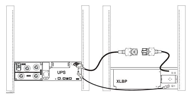
One UPS and one external battery pack and external battery pack battery/communications extension cable connection. See "Connections" on page 2 to secure the five meter battery/communications extension cable connector to UPS/XLBP and secure the ground cable connections.
