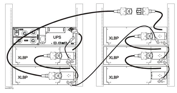
One UPS and five external battery packs and external battery pack battery/communications extension cable connection. See "Connections" on page 2 to secure the five meter battery/communications extension cable connector to UPS/XLBP and secure the ground cable connections.
