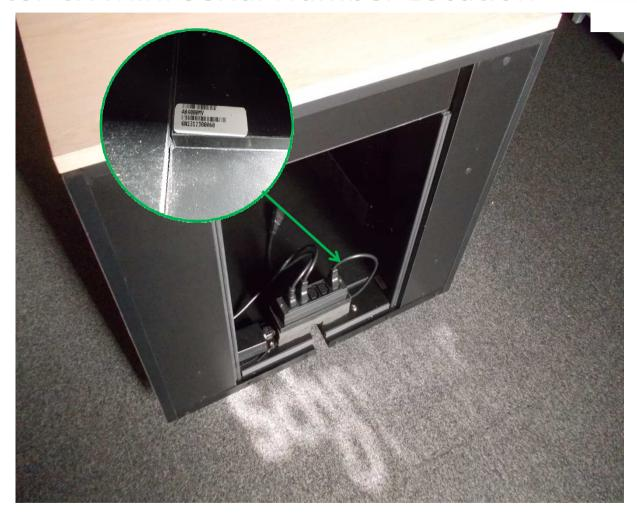
Looking into the <u>rear</u> of a AR4000MV, on the bottom right hand side of the cabinet next to the PDU you will find a small white label adhered to the bottom panel.
