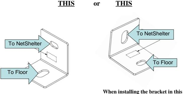
When installing the bracket in this orientation the castors must be removed.
