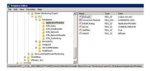
The database connection string information are contained in the keys ION\_Data, ION\_Network, ION\_SystemLog and ApplicationModules. Four keys, one for each database. Each key has 4 values: Server, Initial Catalog, Timeout and Userld. The ApplicationModules key has an additional value 'UseMars'
