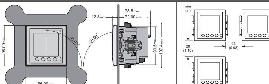
**en** Minimum clearance between mounted meters
