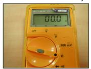
b) If you have an infinite value you are facing an open coils circuit
