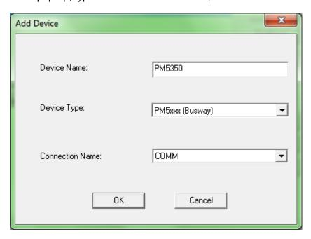
In the next window, under "Rt <u>3</u>" set the "Address" of the connected device, select other values as shown and click "OK":
