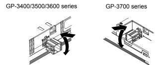
(3) Insert the USB cable into the USB Host Interface.
