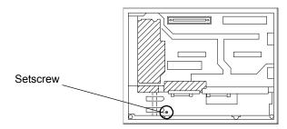
(5) Open the circuit board chassis, lifting from left to right.
