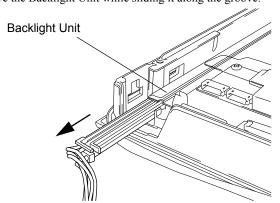
(9) Insert a new Backlight Unit while sliding it along the groove.
