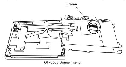
(7) Insert the Function Expansion Memory at an angle so it's base plate locks on to the frame's tabs. While pushing the Function Expansion Memory in the tab's direction, connect to the push-in connector.
