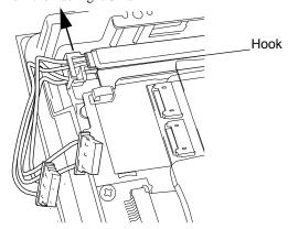
(8) Remove the Backlight Unit while sliding it along the groove.
