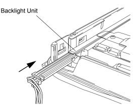
(10) Insert the Backlight Unit cable to the connector on the inverter board, and the secure the cable with the cable clamp.
