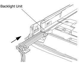
(10) Reattach the backlight unit's setscrew. The necessary torque is 0.196N•m.
