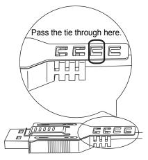
(3) As shown, pass the tie through the clip hole. Next, turn the tie and pass it slightly through the head so that the USB cable can pass through the center of the tie loop. The clip will be lightly attached to the USB cable.
