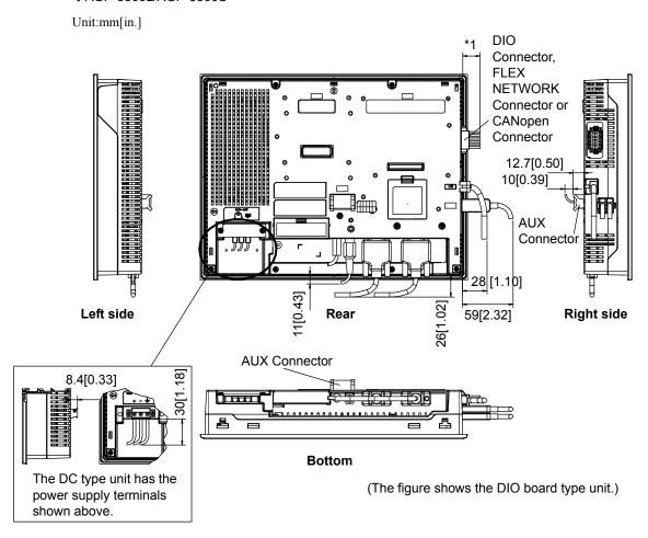
\*1 A 20 mm-space is necessary for the DIO/FLEX NETWORK board and a 127 mm-space for the CANopen board type.
