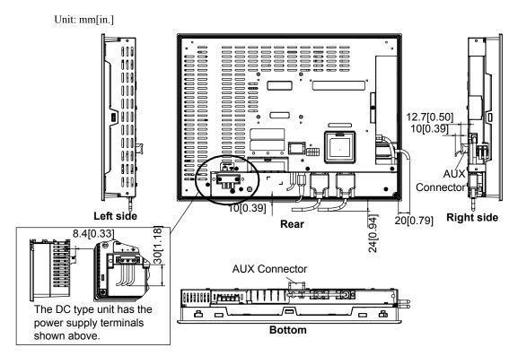
• All the above values are designed in case of cable bending. The dimensions given here are representative values depending on the type of connection cable used.
