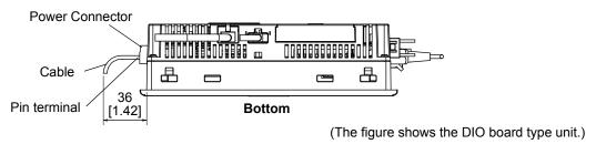
\*1 A 20 mm-space is necessary for the DIO/FLEX NETWORK board and a 127 mm-space for the CANopen board type.
