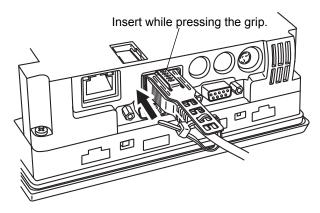
(5) As shown, completely tighten the tie and thoroughly attach the clip on the connector shell.
