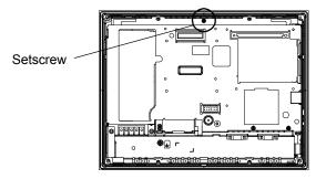
• The Setscrews are not attached to all DC model of GP.
