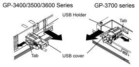
(2) After removing the USB cable, remove the picks pushing the USB Holder from both top and bottom.
