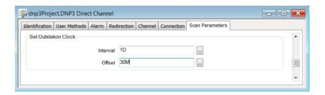
If *Outstation* is selected from the list box, then ClearSCADA will rely solely on the RTU to request the time at the interval set by the *Time Update Request Rate* parameter set in step 1 above.
