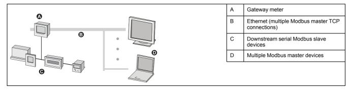
A Modbus master device (such as an energy management system) can communicate through the gateway meter to a serial network of devices connected to the gateway meter's serial port(s). The meter receives Modbus TCP/IP data on
