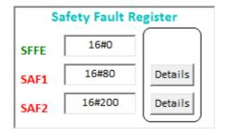
This issue appear mainly when drive is used close to 0Hz (or with high number or Start / stop order). On speed area close to 0, IGBT state checking between Application part and motor control are not synchronized. So drive detect incoherence of signal because they are not synchronize.
