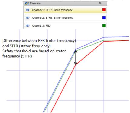
Like you see Rotor frequency (RFR) and Stator Frequency (STFR) are different. We have the slip between both values.
