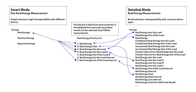
You can select **Detailed** to change to the detailed selection mode. This mode allows you to select from a full list of measurements.
