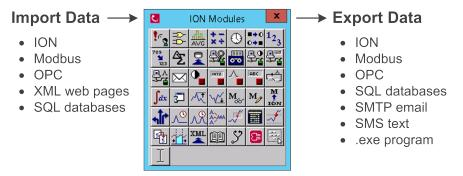
For additional information regarding the configuration and operation of the Virtual Processor of Power Monitoring Expert, see the *StruxureWare Power Monitoring Expert User Guide* and the *ION Reference*.
