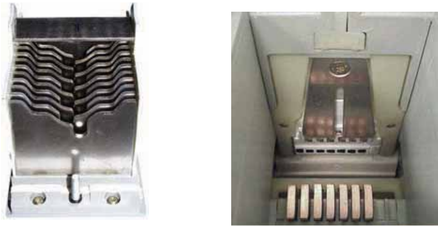
Figure 7 – Wear on Contacts
