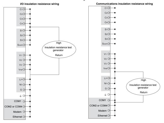
NOTE: Test wiring should be minimum 0.33 mm<sup>2</sup> (22 AWG) or thicker.
