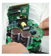
2. Disconnect the connector from the lower power supply board. Do not pull on the wires.
