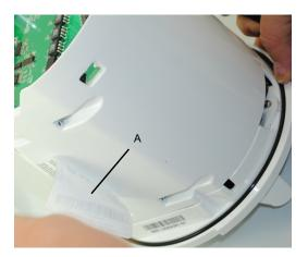
3. Remove the meter side case cover to expose the meter boards.
