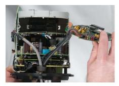
Step 5: Removing and replacing the power supply boards
