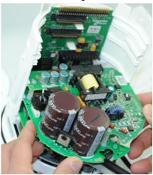
4. Connect the power supply connector to the lower board of the power supply assembly.
