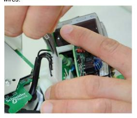
3. Slide the new power supply assembly back into the meter housing and press to insert the board edge connector into the meter connector.
