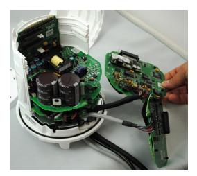
1. Slide the power supply assembly (top and bottom power supply boards) out of the meter.
