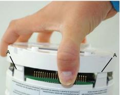
4. Insert the new display board, ensuring proper orientation with the connector on the CPU. Push down on the display board until the tabs click into place.
