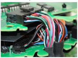
3. Gently slide the new I/O board back into the meter housing and press to insert the board edge connector into the meter connector.
