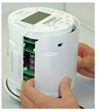
4. Replace the four #2 Phillips screws in the meter side case cover and tighten to 1.7 Nm (15 in-lb).
