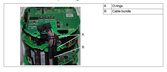
5. Slide the I/O board out of the meter, keeping the cables attached. Position the I/O board to one side to allow access to the inside of the meter.
