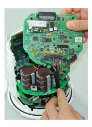
3. Gently slide the communications board back into the meter housing and press to insert the board edge connector into the meter connector.
