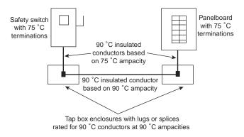
Figure 9: 90 °C Wire Used at 90 °C Ampacity
