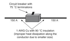
Note: Conductor properly sized based on the termination rating of the circuit breaker.
