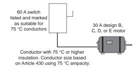
Figure 5: Conductors with Higher Temperature Ratings
