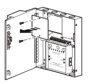
6. Secure the EPO box directly to the junction or switch box with the appropriate number of 6-32 screws around the access window.
