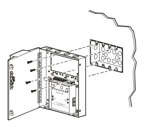
7. Reinforce the EPO box with \(^1/4\)-inch (6.35-millimeter) screws in the corner mounting holes. (See page 14 for a schematic of the EPO box mounting holes.)
