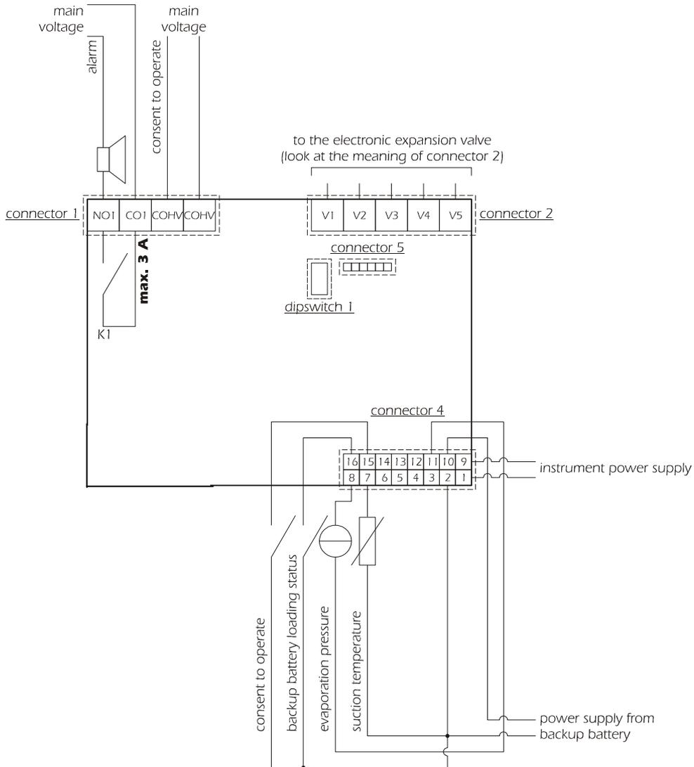
**Connector 1:** functioning consent relay output and digital input (high voltage).
