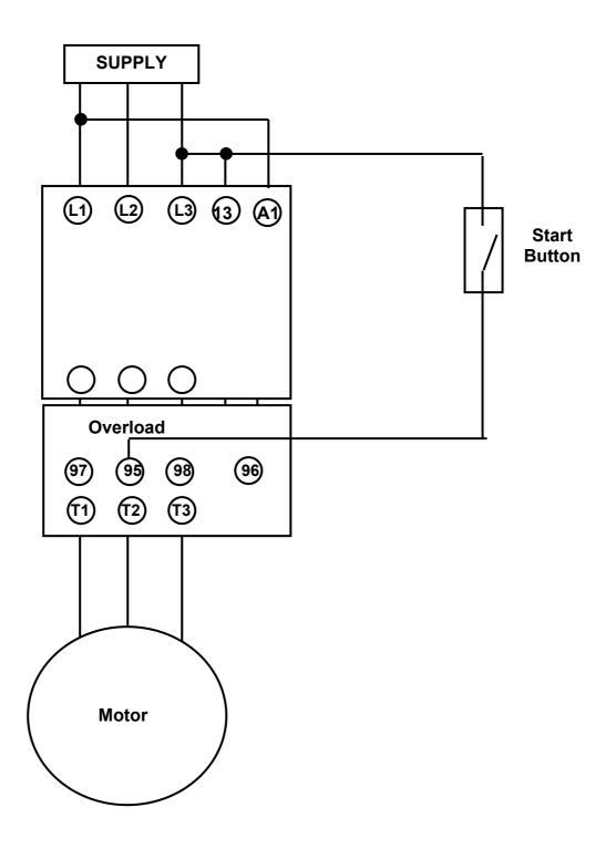
Wiring of K Series DOL starter with 415V coil
