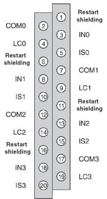
INx + Pole input of channel xCOMx - Pole input of channel xISx + Pole supply of the probeLCx Line compensation
